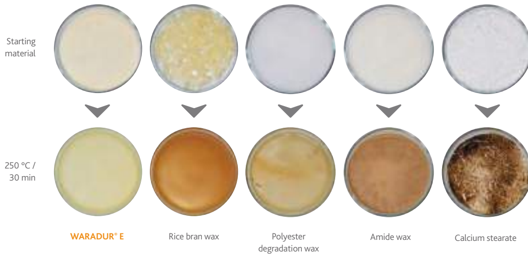
Figure 1: Colour stability under thermal stress (Laboratory Air Circulation Oven Heraeus UT 6120; 250 °C/30 min)
